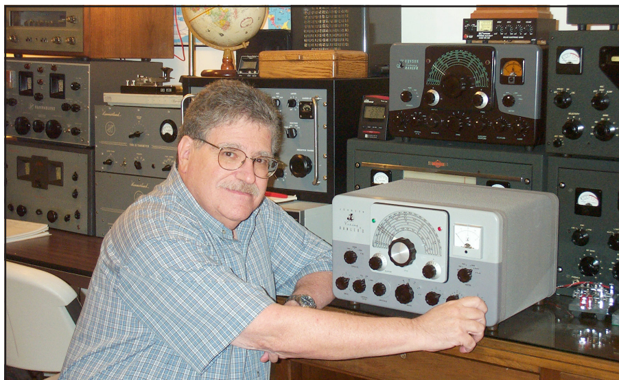
Fig 2.16 — A classic vintage amateur station. The transmitter in the foreground is a Johnson Viking Ranger II. An original Ranger I can be seen above it, to the rear. Classic Collins equipment is below the Ranger I and several Hammarlund receivers and transmitters are on the left.
