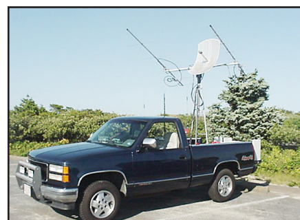
Fig 2.10 — A portable, all purpose, mode V/U/S earth station. This station works LEOs and HEOs (high earth orbiters) like AO-40, and future birds like Eagle. If you live in an area of dense tree growth that impedes your antenna performance, you might consider portable operation at a location with a very low horizon. (photo courtesy of Shawn Reed, N1HOQ).
