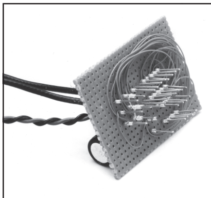
Fig 8.17—The audio amplifier built using wire-wrap techniques.
