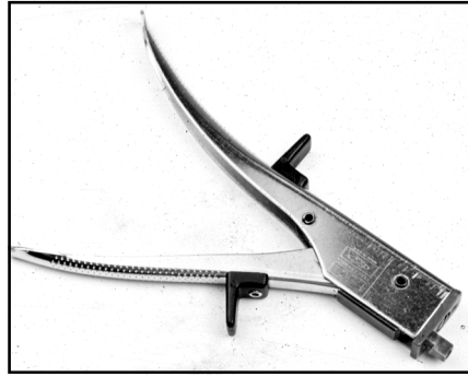
Fig 8.1—A nibbling tool is used to remove small sections of sheet metal.
