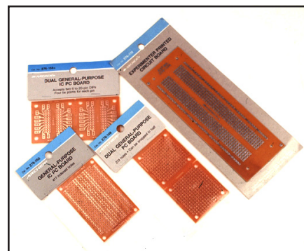
Fig 8.22 —Utility PC boards like these are available from many suppliers.
