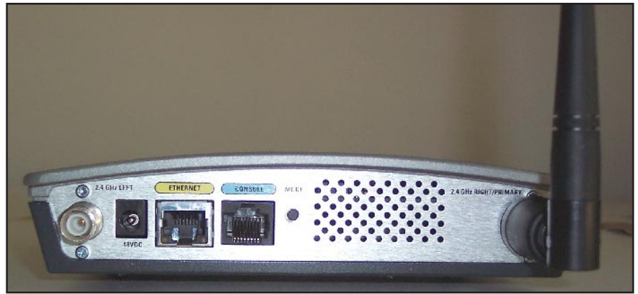
Fig 9.60—Back panel of a typical HSMM-style repeater. This device is known commercially as a wireless access point (AP). It is essentially a computer wireless network hub to enable multiple radio stations to share the various resources of the network. This particular model is a Cisco Model 1200. Note that the left, or secondary antenna's rubber duck has been removed from the TNC connector to show that the connector is of the reverse polarity (RP) type. This is designated as a female TNC/RP connector. Manufacturers of 802.11 gear typically install a RP-type of some type connector to prevent FCC Part 15 unlicensed users from employing their equipment in a non-certified manner. Of course, this is not an issue for licensed Part 97 users, however as in this case, a male RP-type plug will be required in order to connect the device to an outside antenna. The provision of a secondary antenna is to provide space diversity, which helps reduce the negative impact of multipath propagation of the radio signals. The secondary antenna may be ignored when connecting the primary antenna to a single outside antenna, especially if it is a highly directive antenna, which would help reduce multipath effects. (Photo: John Champa, K8OCL)
