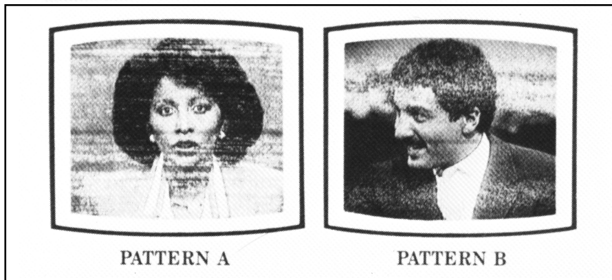
Fig 13.15 — Two examples of TVs experiencing electrical noise.
