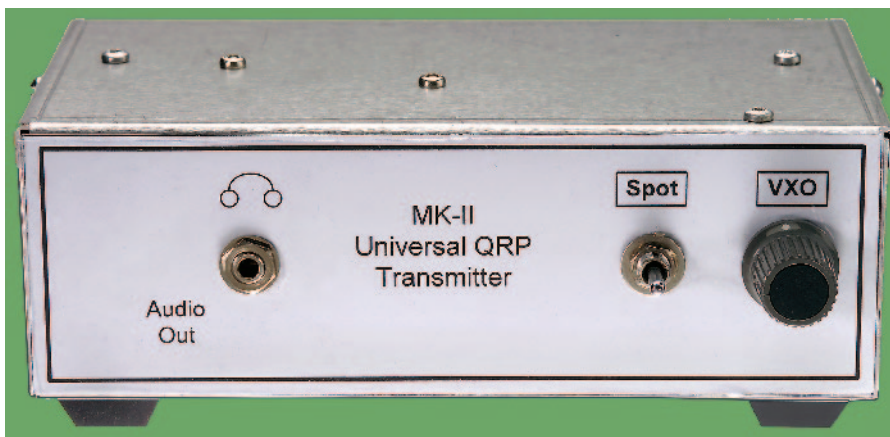
Fig 14.71 — The MKII QRP transmitter includes VXO frequency control, TR switching and a sidetone generator.
