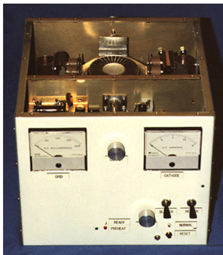
Fig 18.39 —This table-top 2-meter power amplifier uses a quick-warm-up tube, a real plus when the band suddenly opens for DX and you want to join in.
