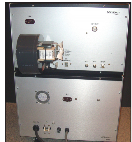
Fig 18.28—At A, front panel view of RF Deck and Power Supply for 3CX1500D7 amplifier. At B, rear view of RF Deck and Power Supply.
