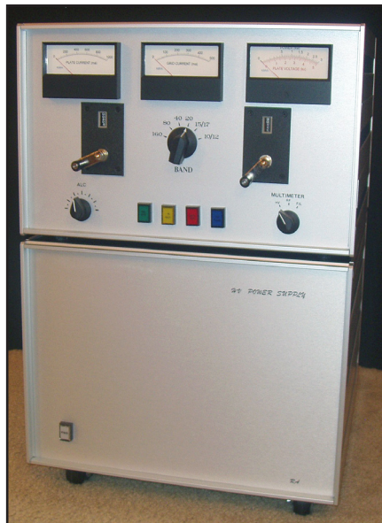
Fig 18.28—At A, front panel view of RF Deck and Power Supply for 3CX1500D7 amplifier. At B, rear view of RF Deck and Power Supply.
