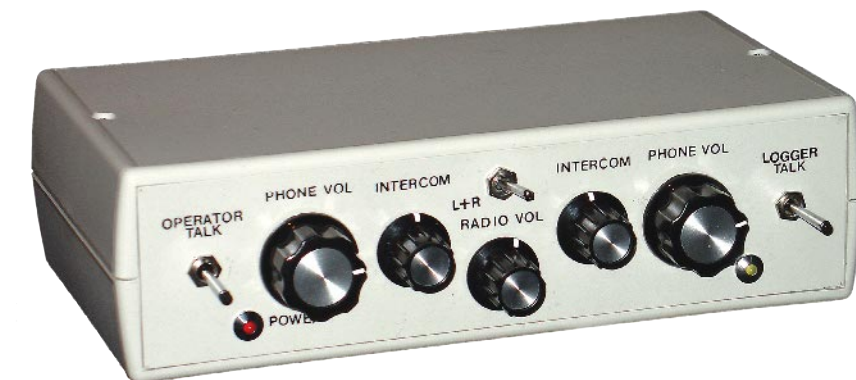
Fig 19.70 — Front view of the audio interface box. Operator controls are on the left and logger controls are on the right.
