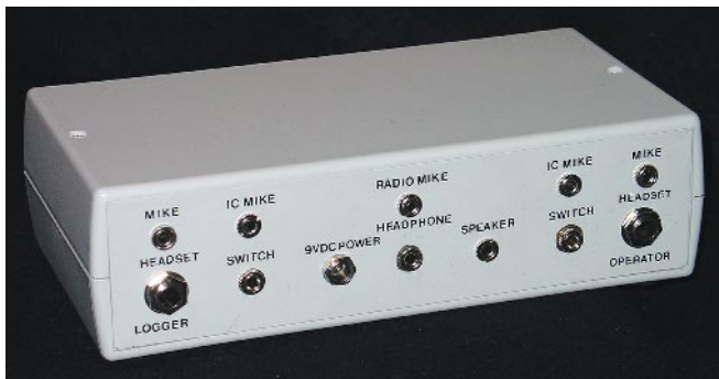
Fig 19.72 — Rear view of the audio interface box. Operator jacks are on the right, logger on the left. Connections to the radio are in the center.
