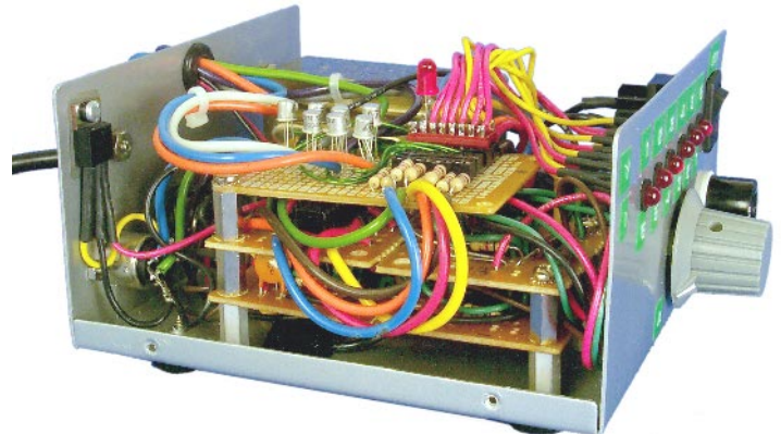
Fig 19.51 —This photo shows the external relay box. The LM7812 regulator is mounted to the bottom of the box. The relay normally open and normally closed contacts are wired in parallel using #12 solid copper. Joe Carcia plans to install two additional relays to use this project at W1AW, so he included the extra flange-mount SO-239 connectors when he was drilling holes in the box. Unused SO-239s can be capped off.
