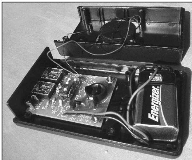
Fig 19.35B — The enhanced EMB version of the TiCK-4 includes a low-current regulator, battery backup and board-mounted jacks and switches.
