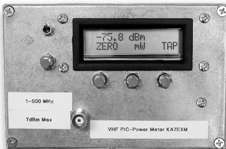
Fig 19.85 — Exterior view of the PIC power meter.
