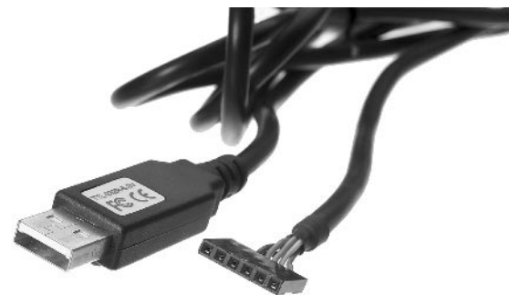
Fig 19.58 — The FTDI TTL-232R cable simplifies construction.
