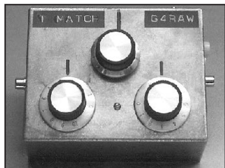
Fig 19.66 —The completed T-Match ATU.
