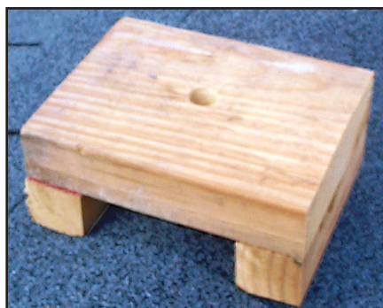
Fig 22.57 — At K8CH, the HVD base insulator sits in this saddle-shaped wooden fixture. This was photo taken before the fixture was painted—a necessary step to protect against the weather.
