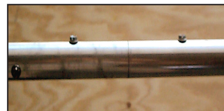
Fig 22.54A — Element splice uses a 1-ft length of 0.75-inch tubing inserted into the 0.875-inch sections to join them together. Self-tapping sheet-metal screws are used in this photo, but aluminum pop rivets or machine screws with washers and nuts can be used.
