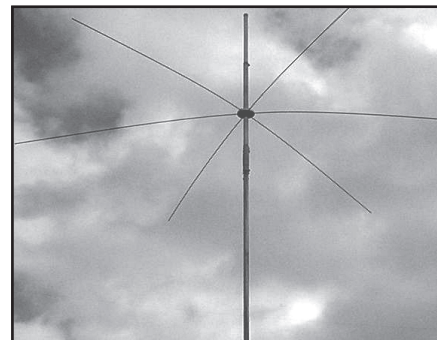
Fig 22.49 — W9SR's short vertical uses top loading and a capacitance hat with a 10-ft TV mast to make a compact antenna for 160, 80 or 40 meters.
