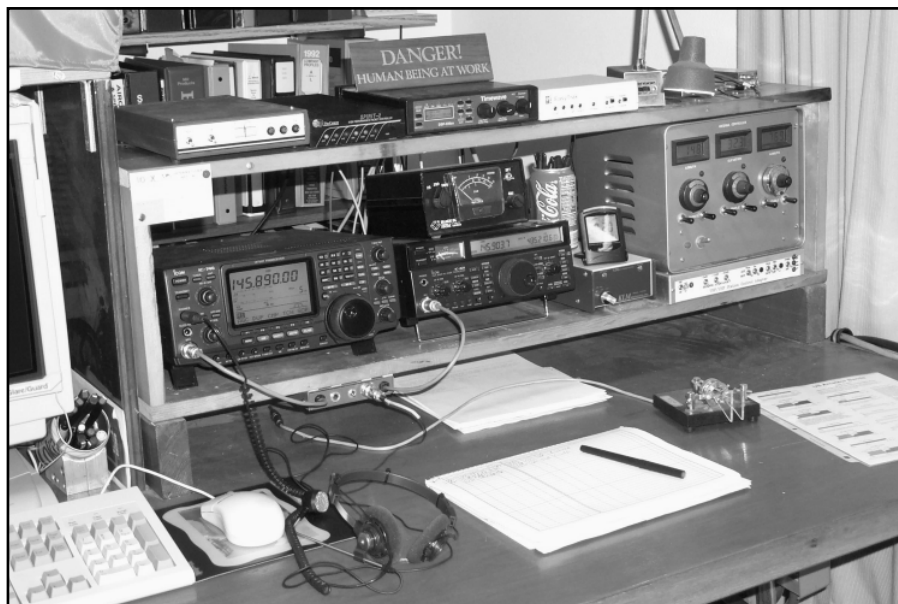
Fig 23.20 —KD1K's station is typical of a full-featured HF and satellite operation. On the bottom row, L-R are: IC-746 HF to 2 meter transceiver, IC-821H VHF-UHF multimode transceiver topped by a home-brew power meter, KLM 1200GU 1.2-GHz transverter, home-brew multi-antenna rotator controller on top of the station accessory control box. On the top row, L-R are: G3RUH AO-13 Telemetry Demodulator, PacComm SPIRIT2 high performance packet controller, Timewave DSP-599zx audio DSP unit for the VHF-microwave operations through the IC-821H and the TAPR EasyTrak antenna command unit for interfacing the computer tracking to the antenna controller.
