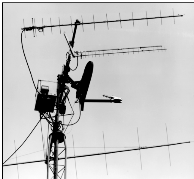
Fig 23.37—Details of KD1K’s tower cluster of satellite antennas, including a home-brew elevation rotator. Top to bottom: M 2 436-CP30, a CP U-band antenna; two each M 2 23CM22EZA antennas shown in a CP array for L band; dish antenna with helix feed for S band; M 2 2M-CP22, a CP V-band antenna (only partially shown.) To left of dish antenna is a NEMA4 equipment box with an internal 40W L-band amplifier, and also hosts externally-mounted preamplifiers.
