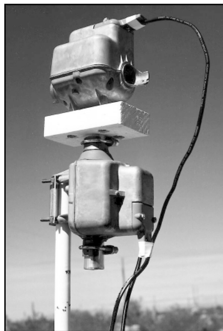
Fig 23.41—VE5FP has a solution for his Az-EI rotators by bolting two of them together in his “An Inexpensive Az-EI Rotator System,” QST , December 1998.
