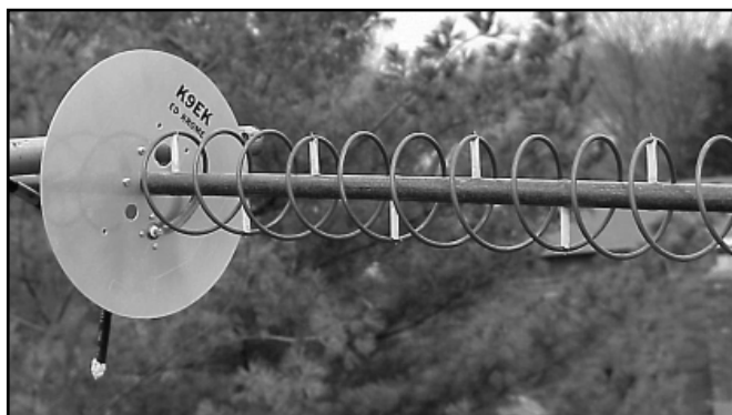
Fig 23.43—This L-band helix antenna was designed to be home-brewed without any special tools or shop equipment. It is mounted on a 4-foot-long fiberglass tube.
