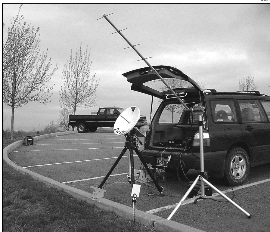
Fig 23.1—N1JEZ's portable microwave satellite station.
