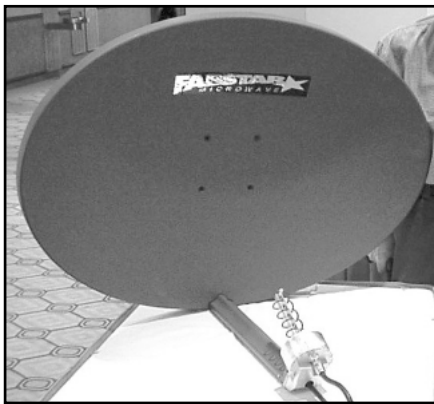
Fig 23.50 —PrimeStar offset-fed dish with KD1K's helix-feed antenna.
