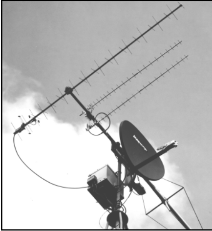
Fig 23.21—Station antennas at KD1K. Mounted are T-B: M2 436-CP30, two stacked M 2 23CM22EZ, modified PrimeStar dish with homebrew seven-turn Helix feed antenna. The M 2 2M-CP22 antenna is off the bottom of the photo. See Fig 23.41 for details of the center section.
