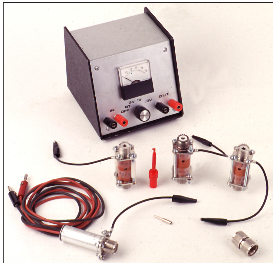
Fig 25.46 — The RF voltmeter with meter unit, RF probe and voltage multipliers.
